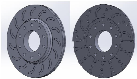
Figure 4: Section View of Segmented Pillar Disc Brake
